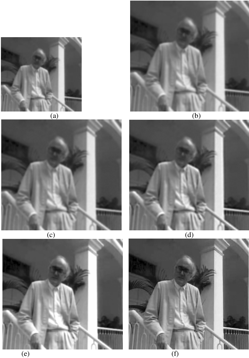
Fig. 2. Actual Video Sequence. (a) the reference LR image. (b) Bilinear interpolation result. (c) POCS estimate. (d) Huber-MAP estimate. (e) HBE result. (f) the HR image.
