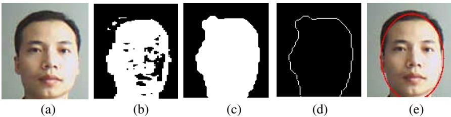
Fig. 5. The realization process of direct least squares ellipse fitting for face. (a) A target region. (b) The skin region. (c) The result of morphological image processing. (d) The face profile. (e) The result of direct least squares ellipse fitting for face.
