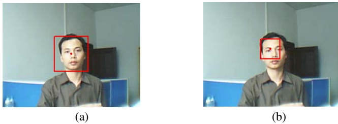
Fig. 3. The demonstration of bandwidth effect for face tracking based on mean shift. (a) The tracking result with a larger scale (bandwidth). (b) The tracking result with a smaller scale (bandwidth).
