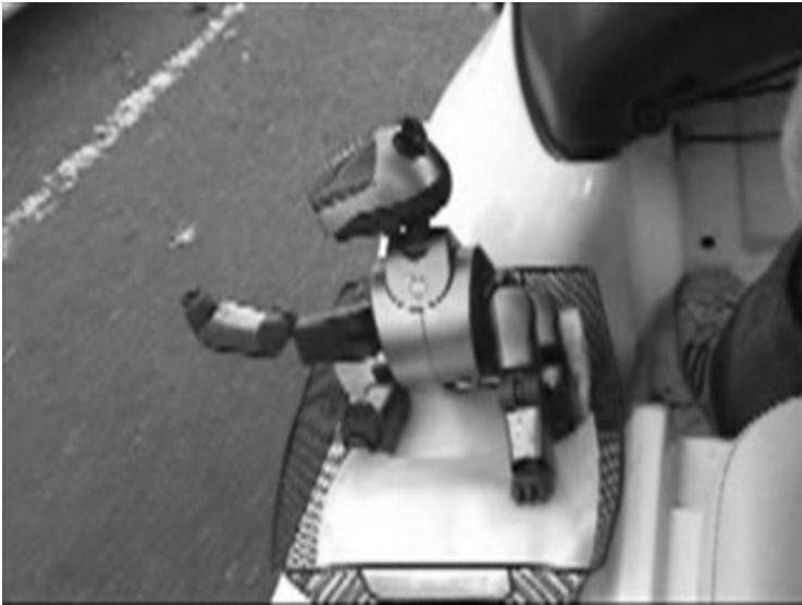
Fig. 4. This image shows Friendly robot's instruction that "there is an obstacle to the left". Friendly robot points to the left of the driver, this means there is an obstacle on the left.
