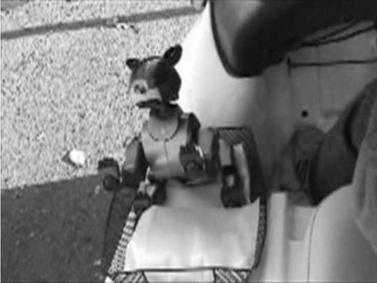
Fig. 5. This image shows Friendly Robot's instruction that "stop". Friendly robot sticks out both hands slowly, this means stop.
