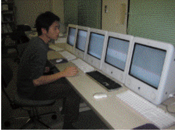
Fig. 5. An example screen of networked mouse experiments with five computers combined with GLIA that realized a 5760-pixel x 814-pixel size workspace
