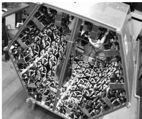
Fig. 1. The hexagonal prism physical implementation of the test-bed, lying on its side with the end open to reveal the cellular internal structure of the electronics
