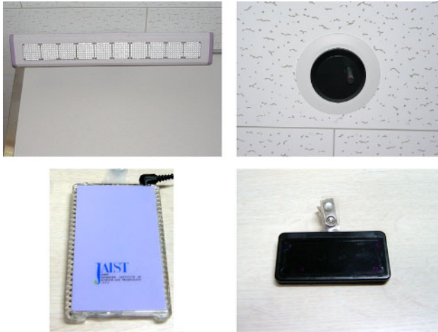
Fig. 2. System devices - Aimulet transmitter (upper-left), optical ID reader embedded in ceiling (upper-right), Aimulet receiver(lower-left), and optical ID badge (lower-right)
