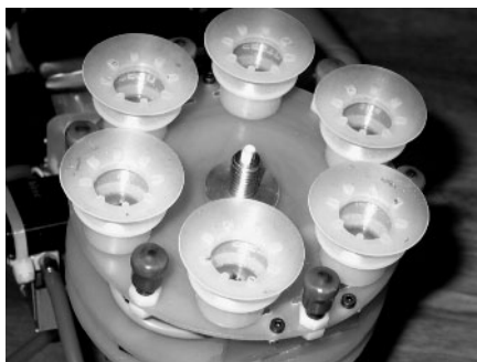
Fig. 5. The ultrasonic communications transducer mounted on the robot foot
