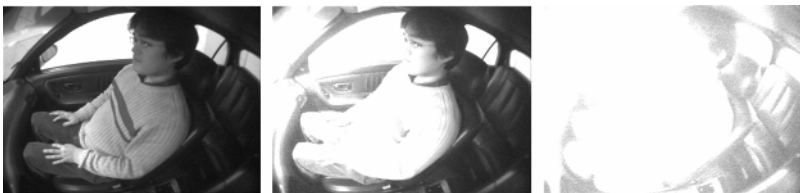
Fig. 3. Camera saturation caused by sunlight or its reflection
