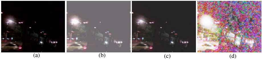
Fig. 5. Applying our proposed algorithm in a night scene with very low contrast (a) Original image. (b) Image enhanced by our algorithm. (c) Image enhanced by global contrast enhancement. (d) Image enhanced by histogram equalization.
