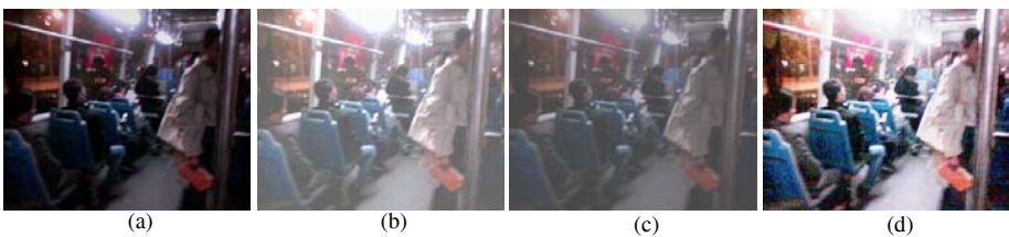
Fig. 4. Applying our proposed algorithm on the bus scene at night with artificial light. (a) Original image. (b) Image enhanced by our algorithm. (c) Image enhanced by global contrast enhancement. (d) Image enhanced by histogram equalization.
