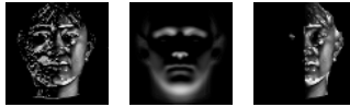
Fig. 4. The first image is the original needle map projected to the x direction of the viewing plane. The second image is the mean needle map that we use as the template. The third image is the needle map projected to the x direction of the viewing plane after the Mean Needle Map Alignment (Sect. 2). The third image compensates the concave/convex problem of the first one.
