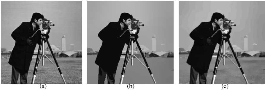
Fig. 3. Cameraman: (a) Original image, (b) Segmented image according to our algorithm hs=12 and hr=15 , (c) Segmented image by using EDISON system hs=8 , hr=4
