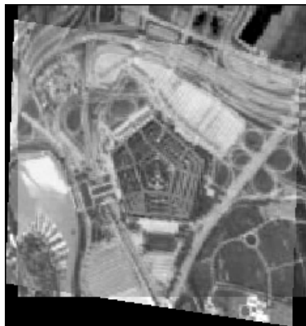
Fig. 3. Registration of optical and infrared images of US Pentagon
