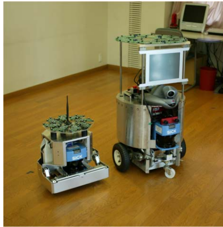
Fig. 1. Mobile Robot Platforms: each with non-holonomic steering and 2D laser range finder sensors
