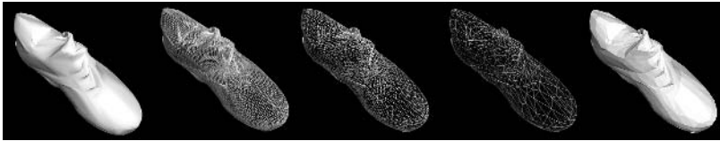
Fig. 11. Illustration of a progressive mesh. From the left to right: the initial model and its mesh, the mesh after one step of simplification, the mesh after two steps of simplification and the model of its mesh after two steps of simplification.
