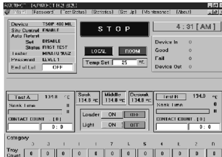
Fig. 6. Main screen of component based control system for IC test handler machine. This system was embedded machine itself. Operator is able to control that machine using this program and receive an operation status message using internet from the other operator at the long distance.
