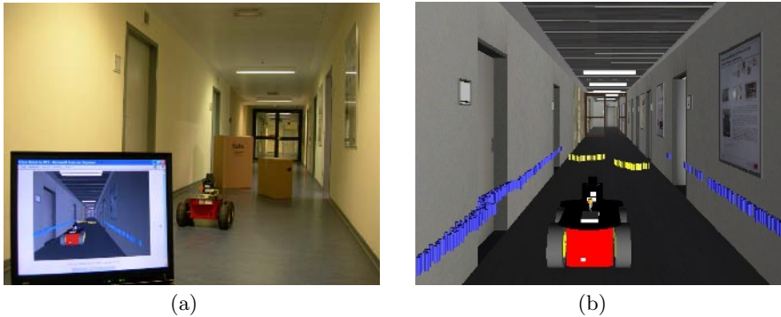
Fig. 4. Robot navigation with a 2D laser scanner (a) A HRI corresponding to the physical navigation environment (b) The HRI shows a MR space where detected objects are highlighted in yellow
