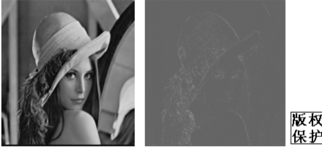
Fig. 4. Left is the watermarked images "Lena" with PSNR=39.34dB and the middle is the absolute difference between original image and watermarked one. Right is the extracted watermark Logo.
