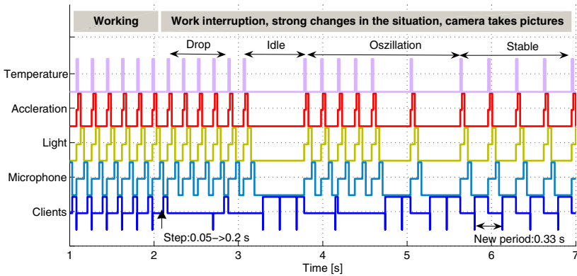
Fig. 12. Scheduling trace of BFS controlled services when situation changes from working to work interruption
