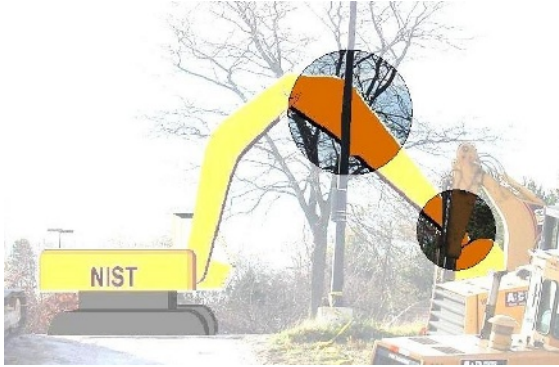
Fig. 6. Dynamic Occlusion Problem in Outdoor Augmented Reality CAD Models Courtesy of Mr. Robert R. Lipman (NIST)
