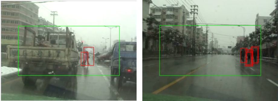
Fig. 8. Pedestrian detection in snowy (left) and rainy (right) weather
