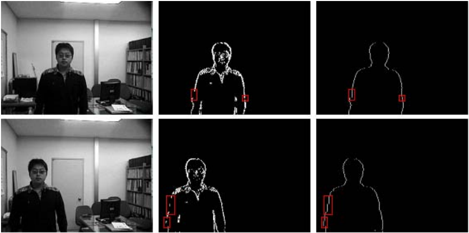
Fig. 2. Original images (left), Differencing images and preprocessed images (center), Edge restoration images (right)
