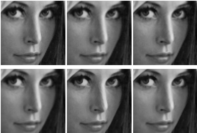
Fig. 2. Enhancing the Lena image (top-left to bottom-right): the nearest, the bilinear, the bicubic, the LSR, the ADSF, and the FFSE
