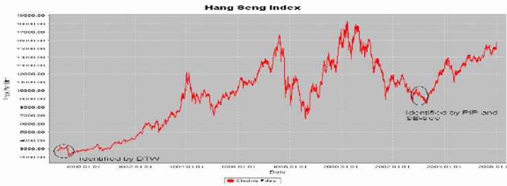
Fig. 11. Sample stock time series (i.e. Hong Kong Heng Sang Index with 4214 data points), the first circled pattern is the query result from DTW method and the second circled pattern is the query result from both PIP and SB-Tree approaches
