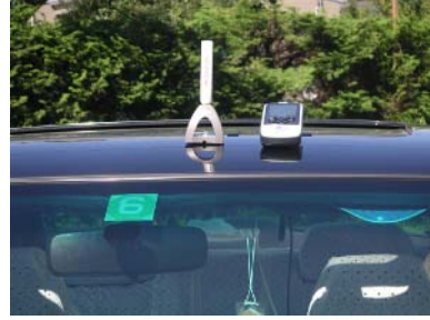
Fig. 5. Left:external antenna Right: GPS device
