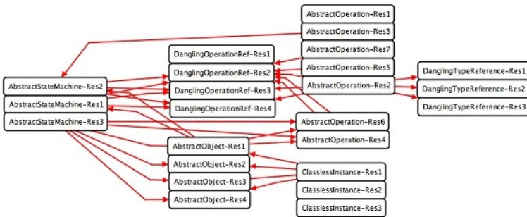
Fig. 6. Graph depicting mutual exclusions between resolution rules of distinct model inconsistencies. Except for some layout issues, this graph has been generated automatically by AGG. In order not to clutter the figure, mutual exclusions between different resolution rules of the same model inconsistency have been omitted.
