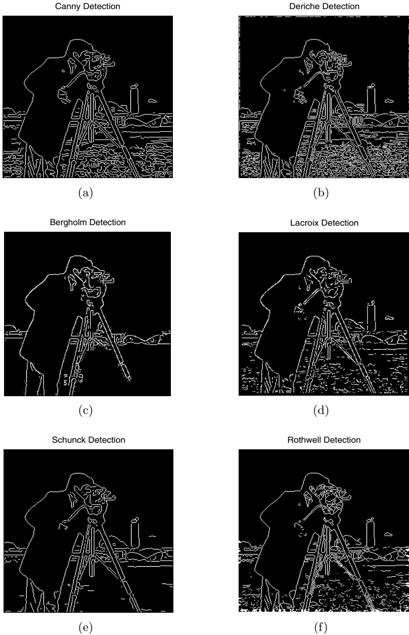
Fig. 2. (a) Canny detection (b) Deriche detection (c) Bergholm detection (d) Lacroix detection (e) Schunck detection (f) Rothwell detection forming the sample set for the Cameraman image
