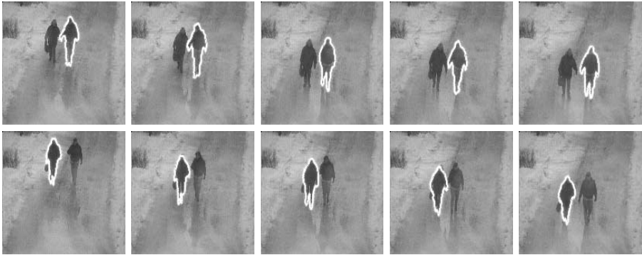
Fig. 4. Tracking results for the Swedish Couple Sequence, using a training set of 7 silhouettes of the man. First row: Tracking the man. Second row: Tracking the woman.
