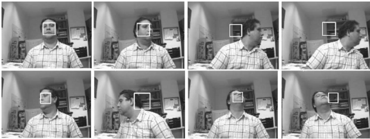
Fig. 4. Face tracking results obtained using only the particle filter. When the detector misses the face, the predicted face is shown at the last detected position.
