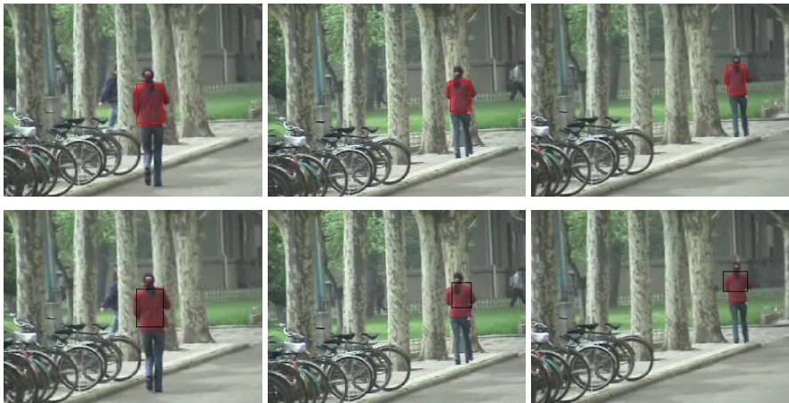
Fig. 5. Tracking results of a pedestrian. Upper row: Using the method presented in this paper. Lower row: Using the bandwidth mean shift tracker. Only the 3 rd , 217 th and 317 th frame.
