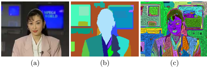
Fig. 2. (a) Input Image. (b) Unconstrained image segmentation used as initialisation. (c) Edge-constrained initialisation of the new regions.
