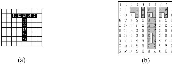
Fig. 4. The mapping pattern M for the secret image “T” using the proposed encoding algorithm (a) the 8×8-pixel secret image with 10 important pixels (b) the 10×10-pixel mapping pattern
