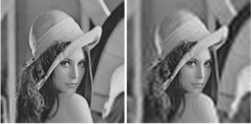
Fig. 6. Fast Hermite foveation with image compression 6 (left) and 12 (right) times
