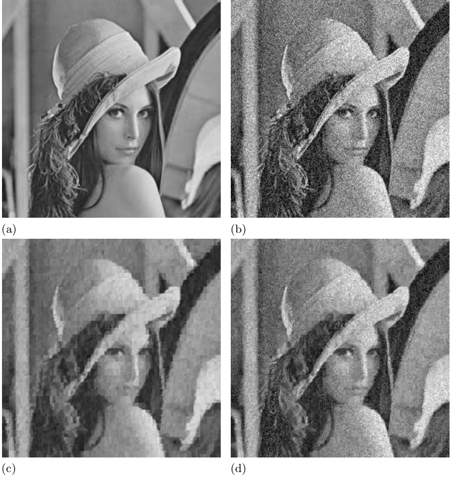
Fig. 3. (a) Lena original. (b) The noisy Image. (c) The IFS attractor of the noisy image, using 8 \times 8 range blocks. (d) Proposed using POCS, the starting point is the noisy image, and the same fractal transform with 8 \times 8 range blocks is used, with \delta = |r|/3 .
