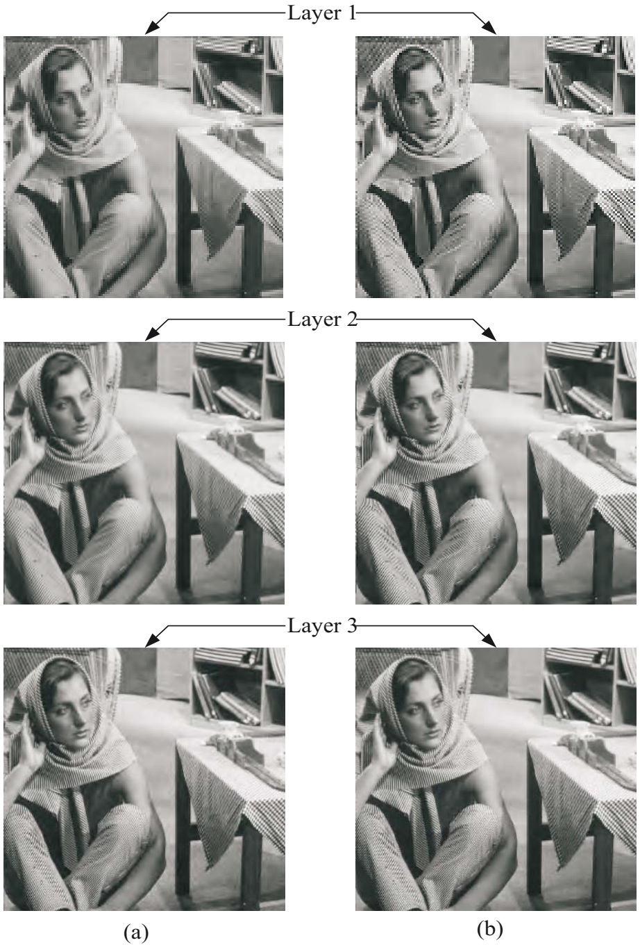
Fig. 5. The reconstructed versions of the image “Barbara” at each layer of LIC systems shown in Table1 : (a): LSPIHT-based LIC system, (b): LJPEG2000-based LIC system
