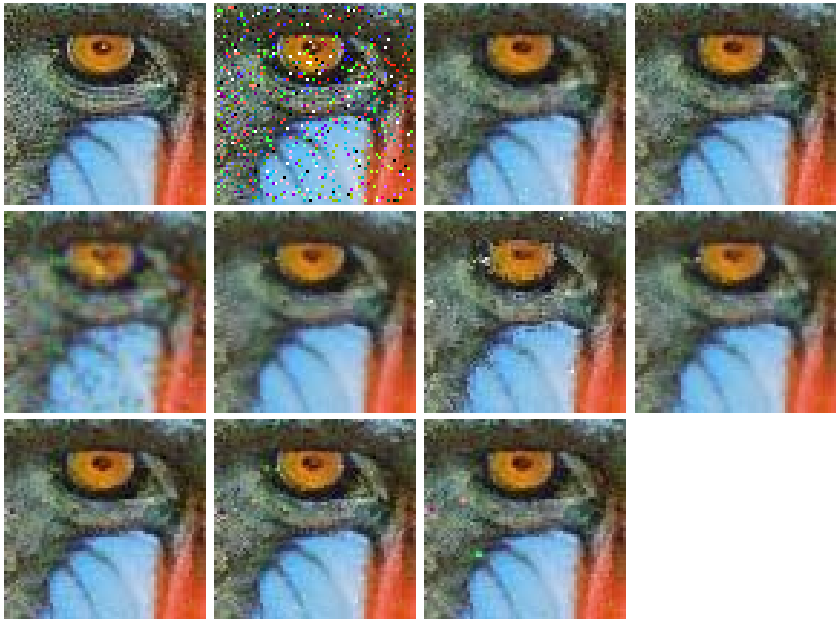
Fig. 2. Results for the Baboon detail image. From left to right and from top to bottom: original image, image with impulsive noise with p = 0.2 , images filtered with: RODSAMF- d^1 , RODSAMF- d^2 , AMF, VMF, BVDF, DDF, FIVF, AVMF, and PGSAMF.
