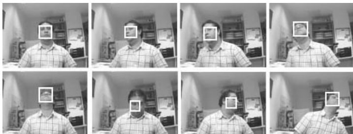
Fig. 5. Face tracking results obtained through the combination of the particle filter and the "CamShift". In this case, no face is missed. The improvements obtained by the use of "CamShift" are obvious.
