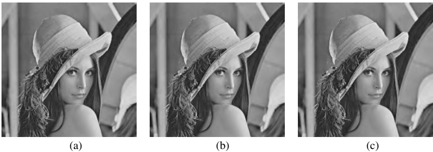
Fig. 4. Decoded images for Lena at 0.25bpp. (a) Variance criterion with GF_0 = 1.075 , PSNR = 34.25dB. (b) L1-norm criterion with CF_0 = 0.935 , PSNR = 34.23dB. (c) R-D optimized cost function (WP-BPO), PSNR = 34.37dB.
