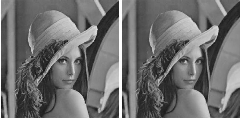
Fig. 5. Left: The limiting image u(x, \infty) produced by integrating Eq. (2) for \epsilon = -0.1 , corresponding to negative diffusion. Euler method, step-size h = 0.001 , integrated to t = 50 . Right: The limiting image for \epsilon = 0 , presented for comparison.
