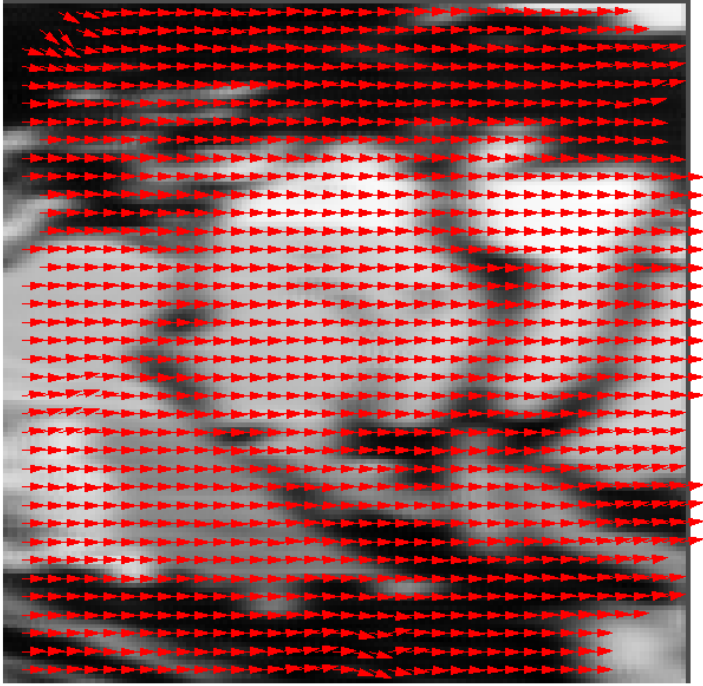
Fig. 3. The estimated flow field of Translating Tree Sequence using time scale \tau = 3 frames
