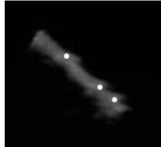
Fig. 6. 3D ultrasound image of a surgical instrument in a water tank with white dots indicating tracked passive markers
