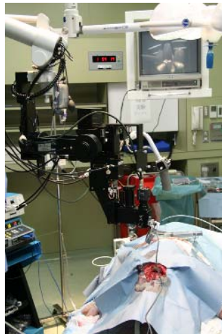
Fig. 3. Automatic focusing and robotic scanning system
