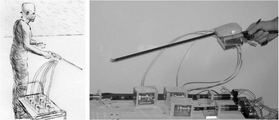
Fig. 1. Concept drawing of the lightweight hand-held laparoscopic robot (left) and the first prototype (right), using the EndoWrist of the da Vinci Surgical System as end-effector
