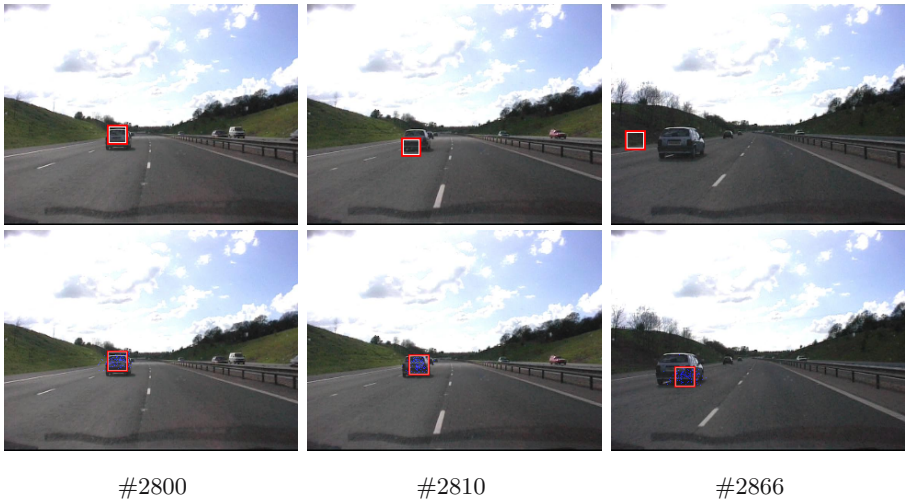
Fig. 4. The results of tracking using CamShift (top row) and particle filter (bottom row)
