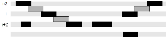
Fig. 8. The segments in dark gray represent the pixels interpolated thanks to the black neighboring segments
