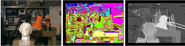
Fig. 1. The Tsukuba image. Left column is the reference view. Middle column is the segment result. Right column is initial disparity map computed by segment cost function.
