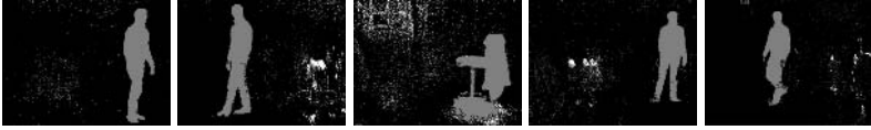
Fig. 2. Examples of extracted silhouettes with the Gaussian mixture model background subtraction technique
