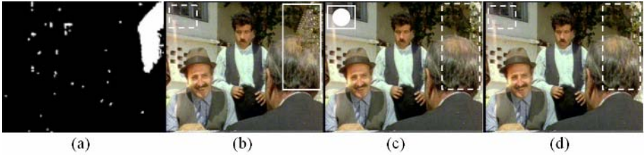
Fig. 8. A sample of the result of restoration of a real corrupted image sequence (frame number 52). (a) Detected blotches, (b) the result of the method presented in [8], (c) the result of the method presented in [7], and (d) the result of the proposed method. The solid rectangles indicate regions in which the restoration has failed, and the dashed rectangles show the regions in which restoration was successful.
