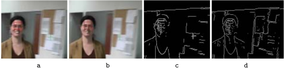
Fig. 6. A frame from Elena sequence: a) Original Image, b) Filtered Image, c) Canny l=170 , h=220 , d) Our approach ( s = 1.0 )
