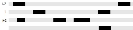
Fig. 4. Example of segments of the same type extracted (in black). The gray lines are known, the white lines are to be interpolated.
