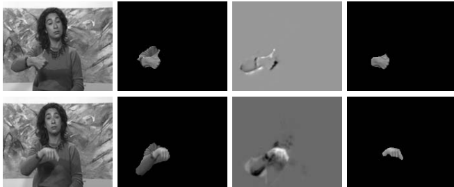
Fig. 6. Two frames of the "silent" sequence: Left: Input data. 2 nd Column: Segmentation using the alternative active model. 3 rd Column: \max(\Psi_{even}, 0) of the selected motion pattern. Right: Segmentation using the composite-feature active model.
