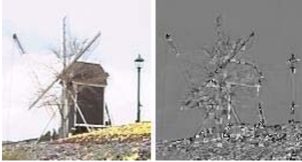
Fig. 1. Part of Flower (CIF) and its residual after intra prediction in H.264
