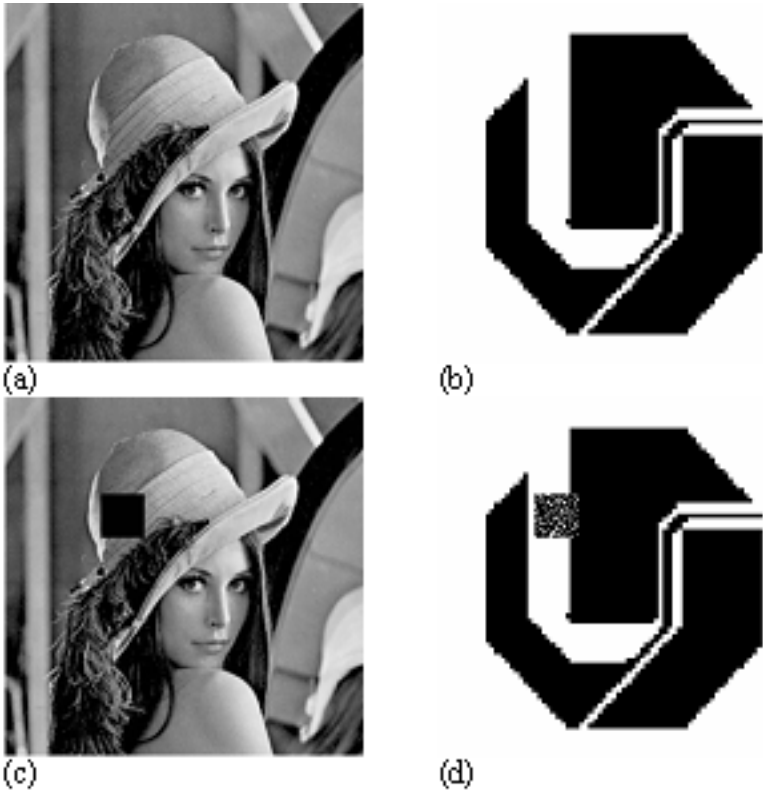
Fig. 2. (a) Watermarked image, (b) Watermark, (c) Attacked image and (d) Extracted watermark
