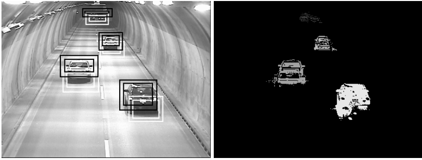
Fig. 13. Left: Image at time t showing the bounding boxes and the considered neighborhood. Right: Blobs classified as foreground.
