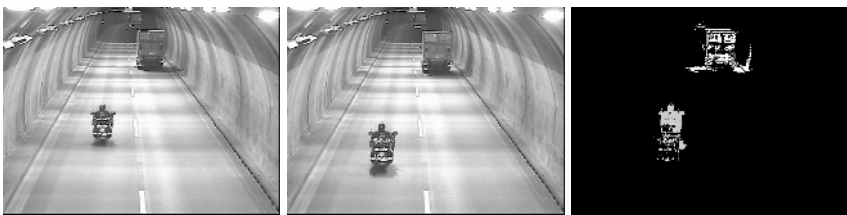
Fig. 14. Left: Image at time t , I_t . Center: Background, I_{(t-1)} . Right: Blobs classified as foreground.
