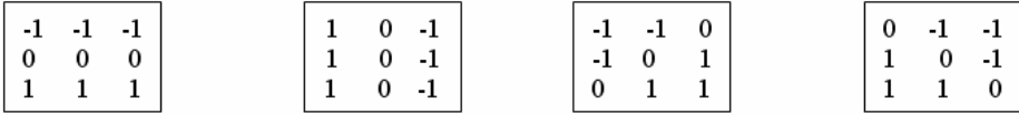
Fig. 1. The convolution masks for component forces on the direction of (from left to right) 90 degrees, 0 degree, 135 degrees, and 45 degrees. The other 4 masks are the transpose of these and we can define the driving force on the opposite direction as negative.
