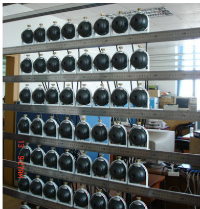
Fig. 7. A photo of our 64-camera light field camera array. The cameras are arranged in rows of eight.
