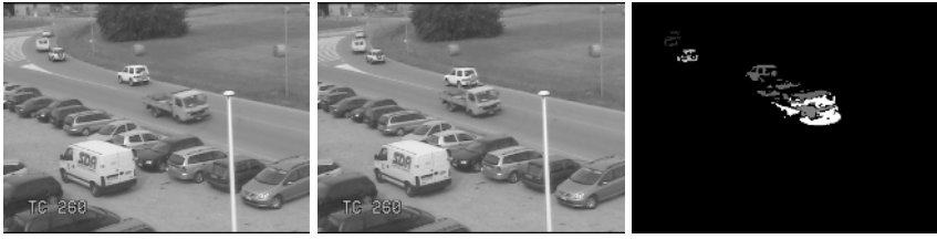
Fig. 15. Left: Image at time t , I_t . Center: Background, I_{(t-1)} . Right: Blobs classified as foreground.
