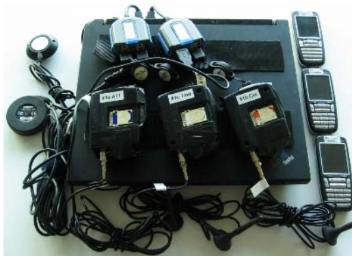
Fig. 1. Our GSM/WiFi data collection device: one WiFi card, two GPS units (left), and three Sony Ericsson GM28 GSM modems (center) are connected to an IBM Thinkpad T30 laptop. The modems require external antennas (bottom) and we have modified them to be powered via USB hubs. Three Audiovox SMT5600 phones, one for each network provider, are shown on the right.
