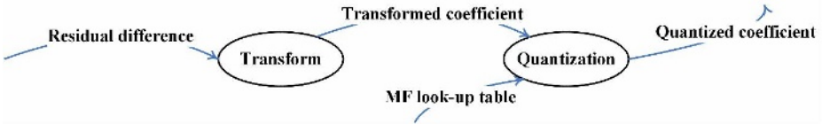
Fig. 3. Kernel diagram. An ellipse represents a computational kernel. And the connection line represents the input or output streams of the kernel.
