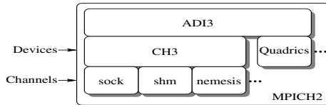
Fig. 1. Software layers of MPICH2
