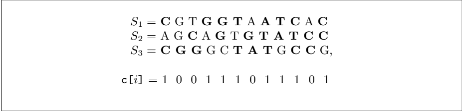
Fig. 1. A genotype in the genetic algorithm and the subsequence that it represents. c[i] = 1 indicates that S_1[i] is in the subsequence, c[i] = 0 that it is not, where S_1[\cdot] is the shortest (or first) of the target instance's strings.
