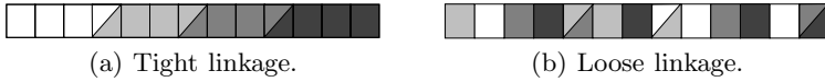
Fig. 1. Examples of ADPs with 4 subproblems of 4 bits each and 1-bit overlap. Each string position (bit) is displayed as a rectangle and the string positions corresponding to one subproblem are filled with the same color. The string positions that are located in more subproblems are split along the diagonal.
