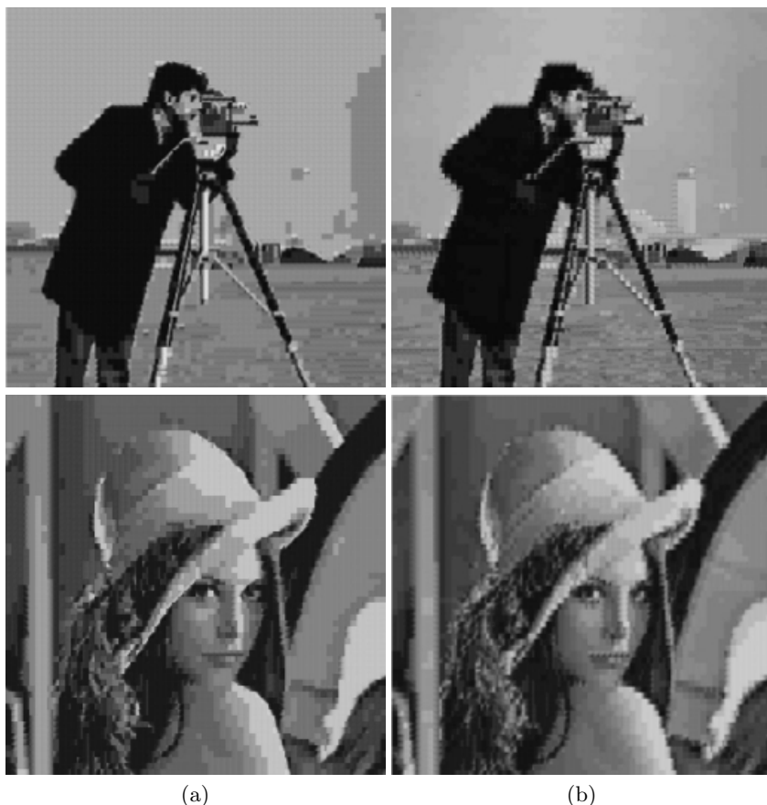
Fig. 2. Compressed test images with L = 4 and K = 32 : (a) by using Standard Competitive Learning (distortions=3.18 and 3.56, from up to down) and (b) by using MREM (distortions=0.67 and 0.81, respectively)
