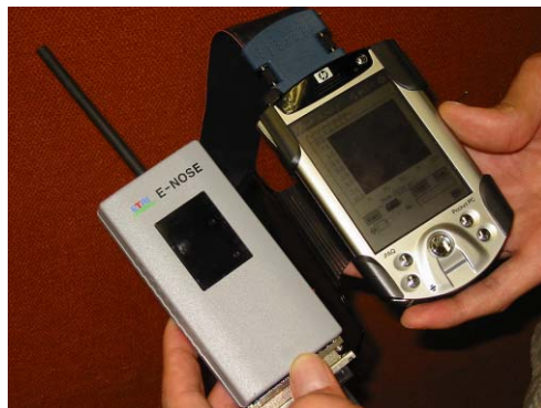
Fig. 3. The developed PDA-based e-nose, a) PDA controls the minimized vapor sensing module via DAQ connection, b) PDA software dedicated for e-nose system displays and stores the measured sensor response
