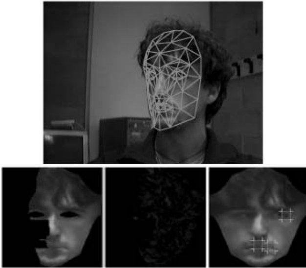
Fig. 2. Examples of face tracking techniques. Starting from the left: self occlusion mask in template (Eyes regions are masked as a very noisy area due blinking and frequent motion), IRLS weight and local feature selection on retrieved face for dissimilarity analysis.
