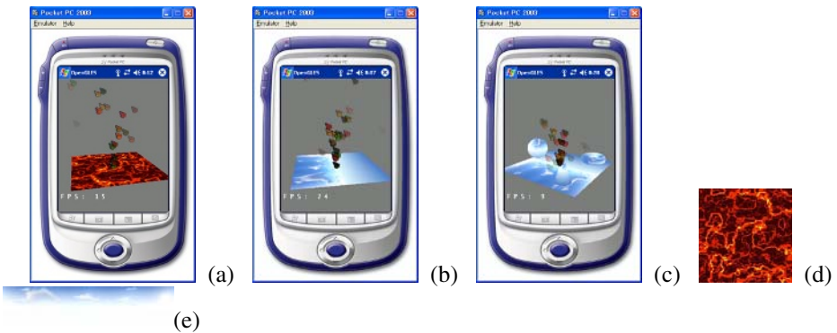
Fig. 5. Result images in a PDA emulator: (a) the image using a mesh file of 102KB and a 64k bytes texture image, (b) the image using a mesh file of 102KB and a 49k bytes texture image, (c) the image using a mesh file of 468 bytes and, (d) a 64k bytes texture image, (e) a 49k bytes texture image
