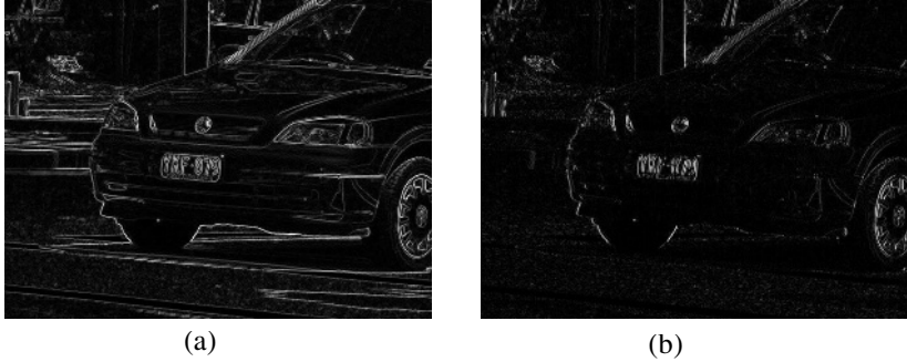
Fig. 2. The gradient images of a image (a) Normal gradient image; (b) Vertical gradient image
