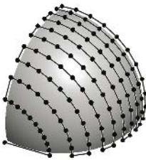
Fig. 8. Directions ordering on 1/8 of the sphere to minimize the exchange of voxels
