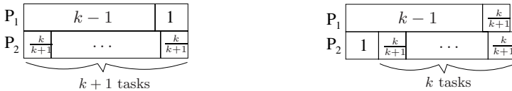
Fig. 3. Left: Optimal schedule for the makespan. This is a k -approximate Nash equilibrium (the policies of the machines are LPT). Right: Approximate schedule for the makespan.
