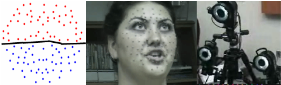
Fig. 1. The left panel illustrates the marker layout used in the objective data analysis. Markers above the solid curve represent markers in the upper face region, and markers below the solid curve are for the lower face region. The middle panel is a snapshot of the record video. The right panel illustrates the used motion capture system.
