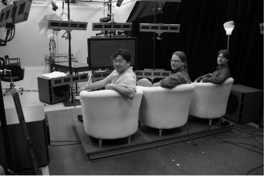
Fig. 1. A photograph of the installation at the Immersive Presence Lab at McGill University. The loudspeaker array, visual display, and motion platform are visible. Three participants (not the individuals shown) sat at the positions indicated.
