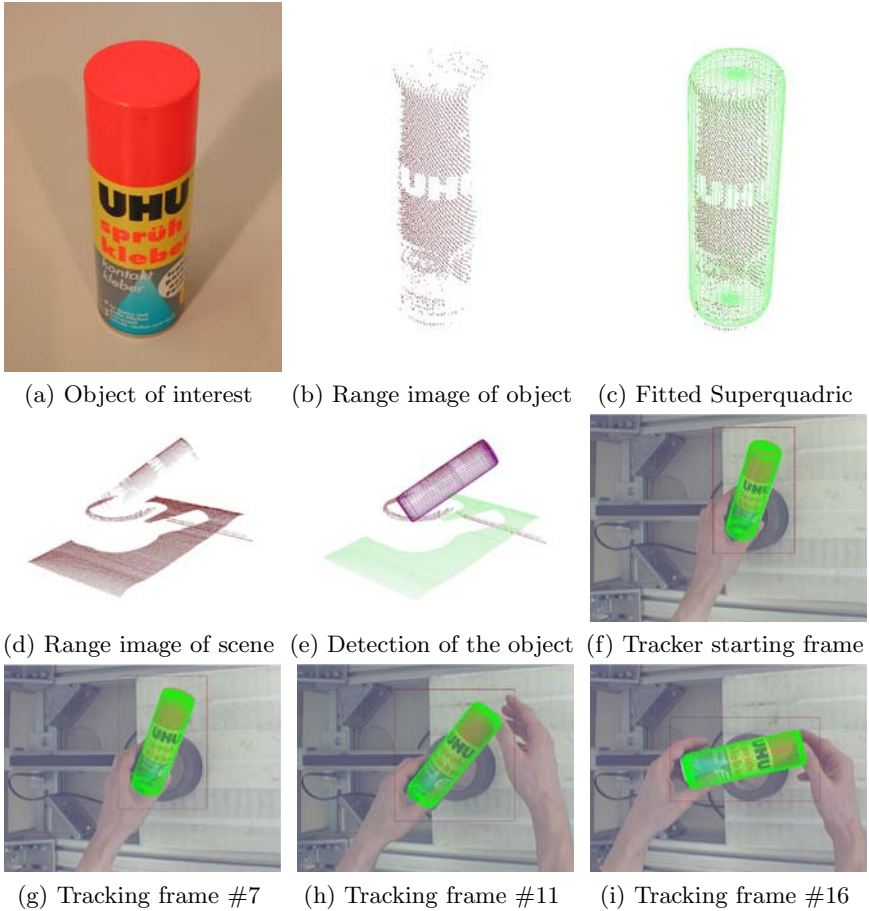
Fig. 3. Experiment 1: Handling of a cylinder. Capturing model (first row), Detecting (second row) and Tracking (last row). The reprojected pose is depicted as mesh-grid.
