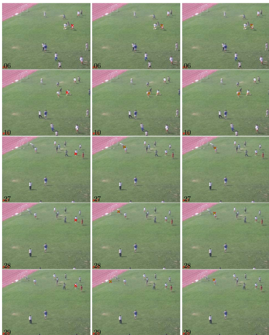
Fig. 8. Tracking results of models fusion layer. The tracked player position estimated is marked with a red cross. The left column displays mean shift only tracking result. The middle column shows the result of Kalman + mean shift method. And the result of our method, pseudo measurement based multiple model approach, is put in the right column.
