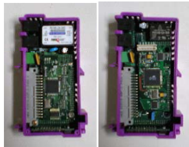
Fig. 3. Slave devices for (a) DIO (b) motion control
