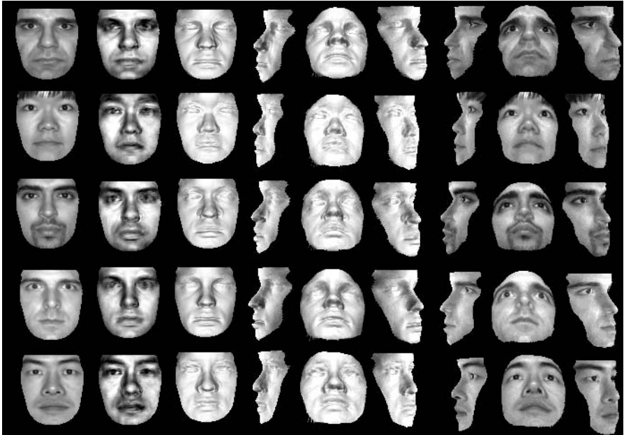
Fig. 4. Height recovery results using five examples from the Yale B database. From left to right: input image, intensity best-fit recovery, frontal illumination of the recovered height and profile and close-to-profile views with warped albedo-free and input images.
