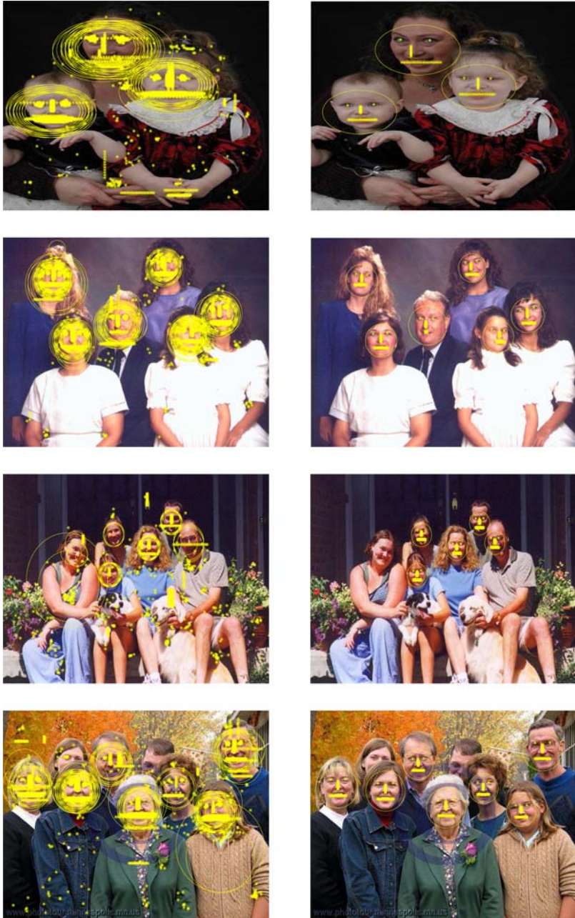
Fig. 5. On the left hand side images the initial unclustered detection results on a number of images is shown. The face detections are indicated by blue circles, the eyes by magenta stars, the mouths by red horizontal lines and the noses by yellow vertical lines. The sizes indicate the scale of the detections. On the right hand side the maximum likelihood estimates of the scenes are shown.
