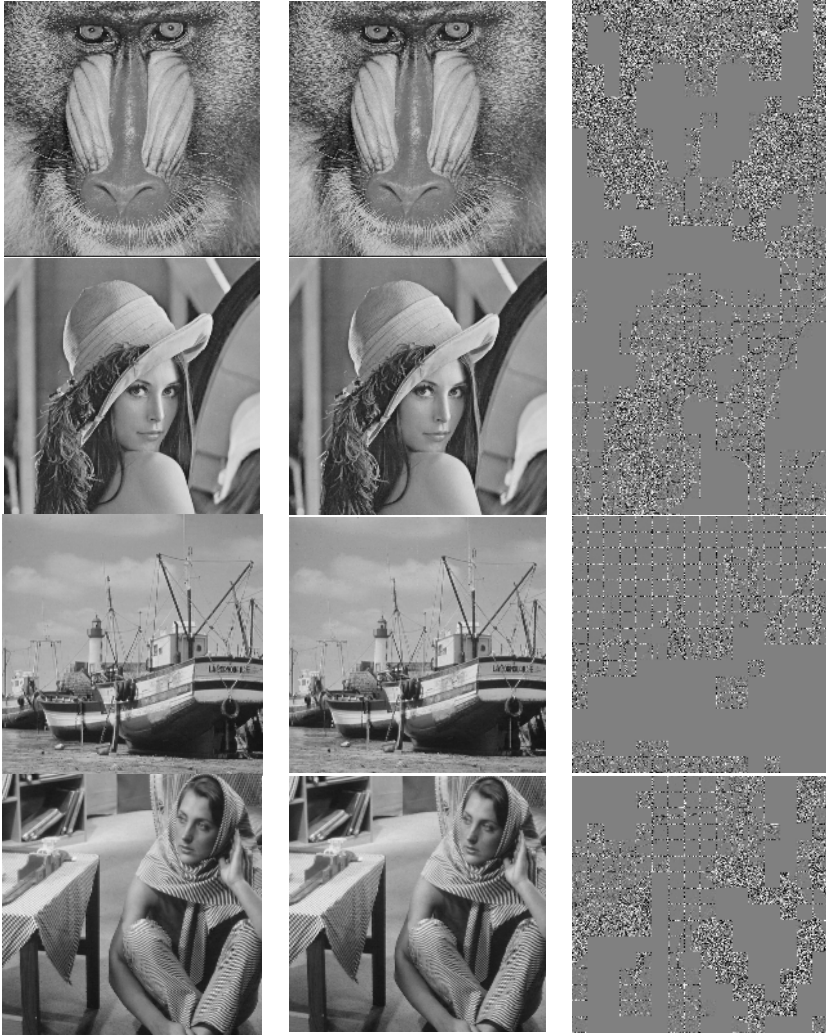
Fig. 3. Fingerprinted images, and their fingerprints (Enlarged), the number of Marks ( M ) =10, Repetition factor ( R ) =16, Block size = 32 \times 32 : (top) Baboon (PSNR: 40.69 dB), (second) Lena (PSNR: 44.07 dB), (third) Boat (PSNR: 45.45 dB), (bottom) Barbara (PSNR: 42.72 dB)
