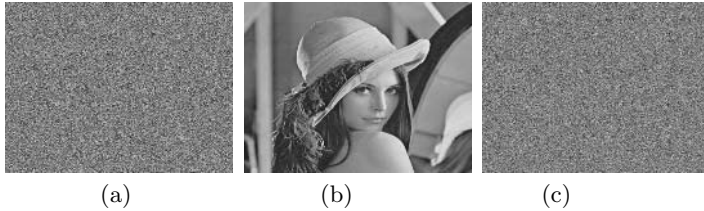
Fig. 4. Key sensitive test: (a) ciphered image encrypted by using key string 'abc123', (b) deciphered image by using key string 'abc123'; (c) deciphered image by using key string 'abc124'
