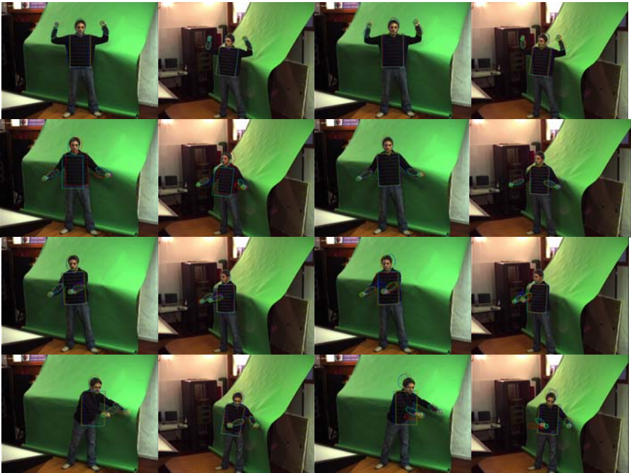
Fig. 6. The first and second columns are computed without biomechanical restrictions from camera \gamma_1 , \gamma_2 respectively. The third and fourth columns correspond to camera \gamma_1 , \gamma_2 and are computed with restrictions. From top to bottom are frames 51, 90, 150 and 250. Last row shows the improvement of biomechanical restrictions, right elbow joint position is right. Our best solution is displayed in green, red are mean solution, and blue are best particle solution.
