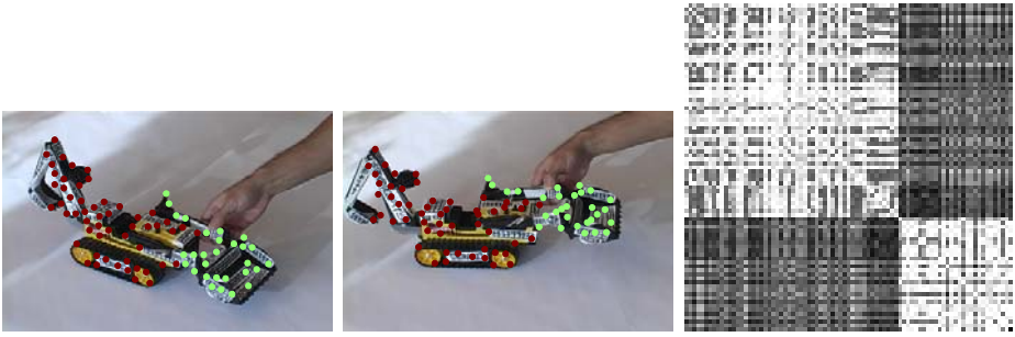
Fig. 1. ( left and middle ) A sequence of a truck moving with the shovel rotating around an axis. The color of a dot, red or green, shows the segmentation result. ( right ) The affinity matrix of local estimated subspaces is shown. The row and columns are rearranged based on the segmentation.
