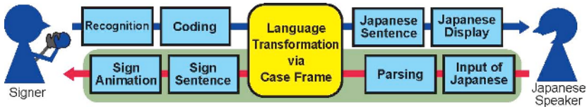
Fig. 1. The system bi-directionally translating between JSL and Japanese. The shadowed part illustrates translation from Japanese into JSL.
