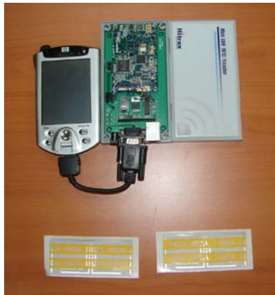
Fig. 1. Overall block diagram of the Blind Interactive Guide System. It consists of a HP 5450 iPAQ PDA, M-200 RFID reader from Hitrax, and tags.
