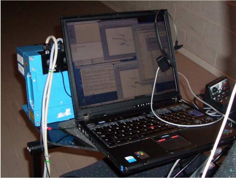
Fig. 2. MultiPos - A head mounted gyroscope used as a mouse interface to a computer. It is visible hanging on the laptop screen. With the gyro interface the user can operate the computer and select a destination for the wheelchair.
