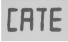
Fig. 7. Word "CATE" written using retractable electromagnetic writing tip
