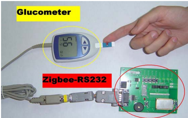
Fig. 2. Sensor connection with the Zigbee module
