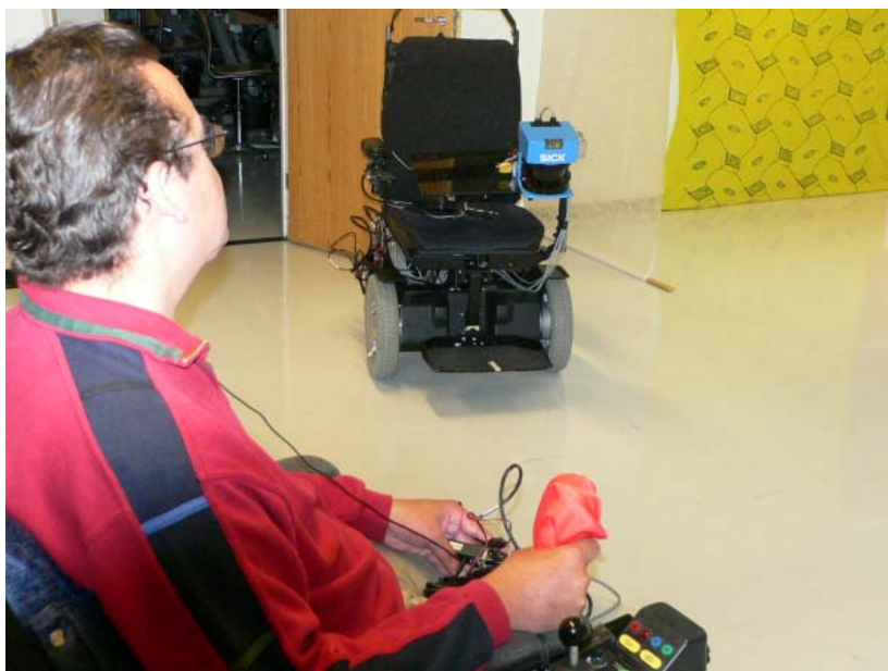
Fig. 1. Mr Tapio Yliruikka, the wheelchair user, holds a steering unit that makes it possible from him to remote control the MICA wheelchair. The range scanning laser is visible on the wheelchair.
