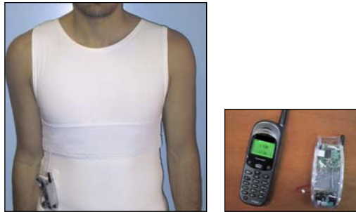
Fig. 4. The sensorized t-shirt and the electronic board. The dimensions of the electronic board are compared to those of a cell phone.
