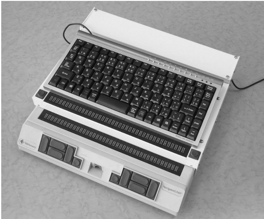
Fig. 1. An overview of Doubled Braille display terminal for the Deaf-Blind person (DB4DB). The Braille array of near side displays all messages from members in a chat space, and another array in back side displays sending message from the user. On the back side of the terminal there are two serial ports to which different control signals are inputted.
