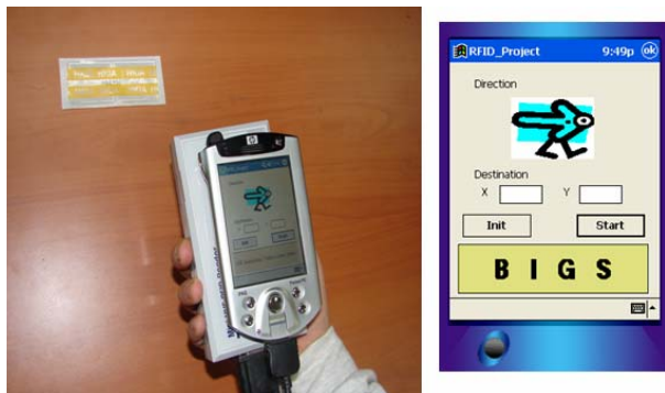
Fig. 6. The user is starting the navigation. In the right picture, the RFID reader is sitting under the 5450 PDA.
