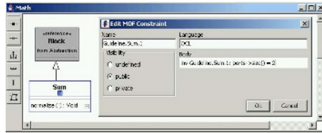
Fig. 5. Design guideline as OCL 2.0 constraint in MOFLON
