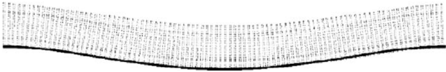
Fig. 24.40. Comparison between MD and beam theory for the deflection of a 20-nm-long fixed-fixed double-walled nanotube (diameter 1.96 nm). The solid black curve is the deflection predicted by beam theory. (Reprinted with permission from Dequesnes et al. [109]. Copyright 2002, Institute of Physics)
