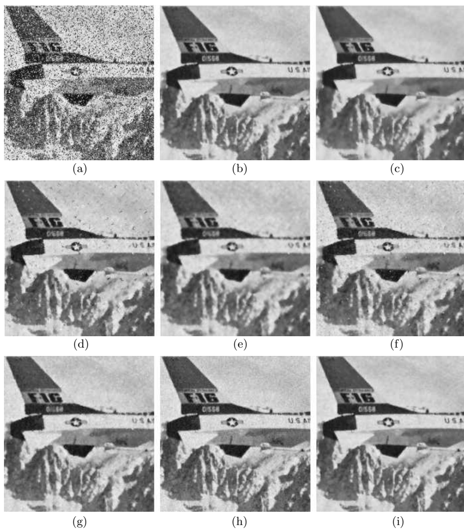
Fig. 2. The corrupted image (a) “Airplane” with 20% impulses and Gaussian noise of \sigma=20 ; (b) FK-NN with Wiener filter; (c) FK-NN with Wiener filter; (d) FWLS [5]; (e) MFF [6]; (f) FLF [7]; (g) PBM [1]; (h) FK-NN; and (i) Two-Stage method
