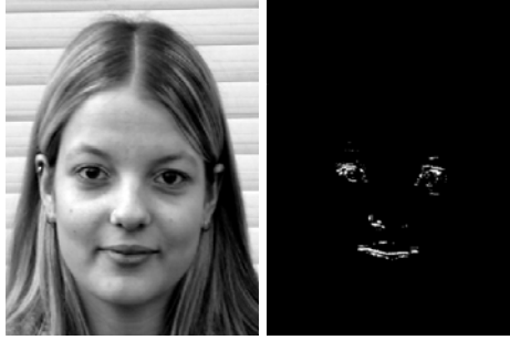
Fig. 6. Original test image "Fadab127" from FaDab Database [3] and the corresponding resulting image ThreshDST(I(x)) with the extracted salient points
