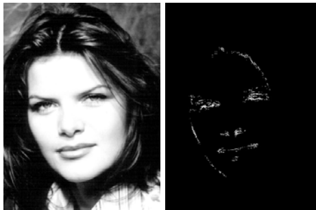
Fig. 7. Original image "Fadab044" from FaDab Database [3] and the corresponding resulting image ThreshDST(I(x)) with the extracted salient points
