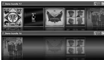
Fig. 7. Demonstration of the complete policy enforcement framework. The system can be used for configuring the Knopflerfish desktop. Each graphical desktop component can be made invisible since each component is a service. The proof of concept implementation does not make the visibility rules persistent across a framework restart, but this could be done easily by saving the persistent service IDs and bundle IDs.
