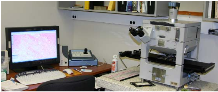
Fig. 2. a) Following CT imaging, the tissue sample embedded in agar was cut into 5mm-thick slabs (breadloafed). Alternate slabs were sent to clinical pathology for a routine work-up. b) The microscope with motorized stage and image display workstation.
