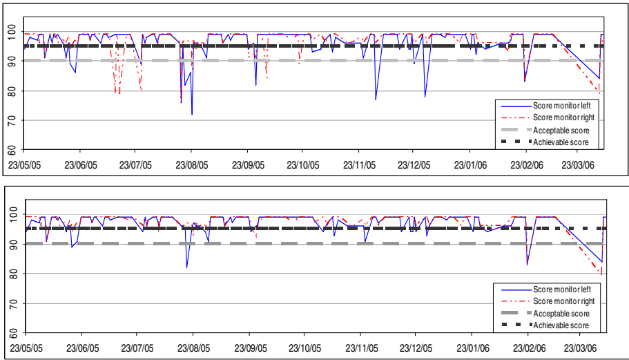
Fig. 3. MoniQA score of two monitors in a dual-monitor setup (workstation A – mammography) with level markers both acceptable and achievable. (top graph) uncorrected score; (bottom graph) corrected score.
