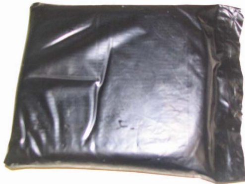
Fig. 2. MREIM phantom made of agar gel and ProHance solution in a polyethelene bag
