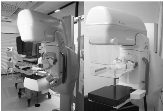
Fig. 2. On the left side Diamond Delta 32 for diagnostic breast tomosynthesis system. This system incorporates a CCD small-area detector with 48 \mu\text{m} pixel size, and is using TACT 3D technology. On the right side the prototype of tomosynthesis FFDM system (Diamond DX) based on a -Se technology with 85 \mu\text{m} pixel size.
