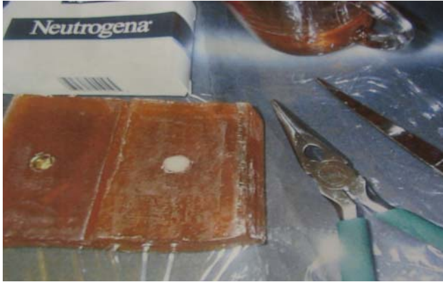
Fig. 1. Sliced MREIM phantom constructed of fragrance free Neutrogena soap showing the spherical piece of fat-free hotdog, 1 cm in diameter, simulating cancer
