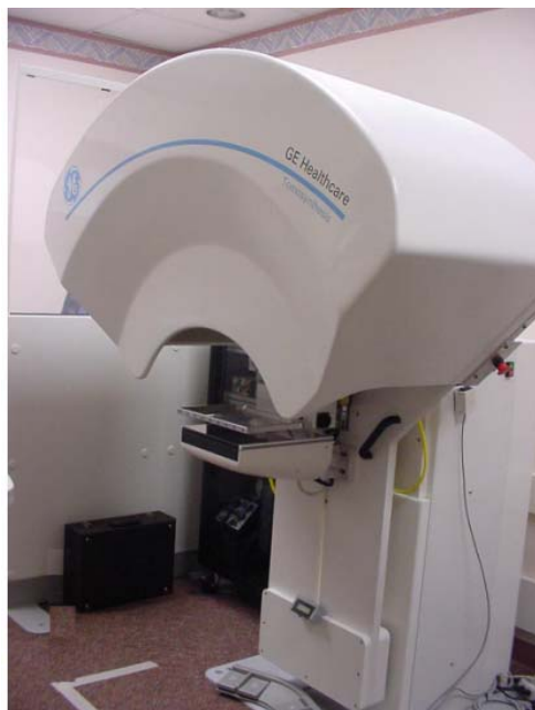
Fig. 2. Photograph of the prototype tomosynthesis system installed at the University of Michigan Cancer and Geriatric Center
