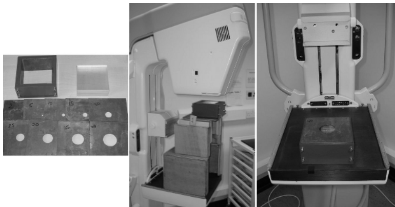
Fig. 3. The experimental setup: the apertures, phantom, and phantom side shielding (left), measurement of the primary beam (centre), measurement of scatter characteristics (right)
