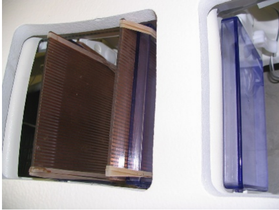
Fig. 3. Photograph of the stabilization/compression paddles of the MR breast coil. The left paddle of the coil was modified to include a Faraday shield made of a pair of copper sheets consisting of rectangular parallel bars. The copper sheets shown here were 14x15 cm. The phantoms were positioned between the two plates for imaging.
