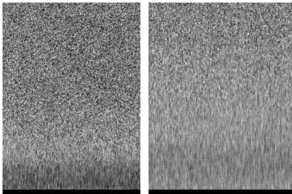
Fig. 3. Crystallization of selenium at lateral side of the detector. The size of the area shown is approximately 3 by 4 cm. a: Image from November, b: Image from January.
