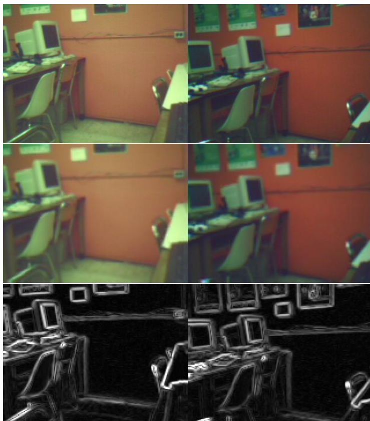
Fig. 1. The product of applying a Gaussian blur (middle) on the raw image pair (top). The blurred image is then subjected to Sobel edge detection (bottom).
