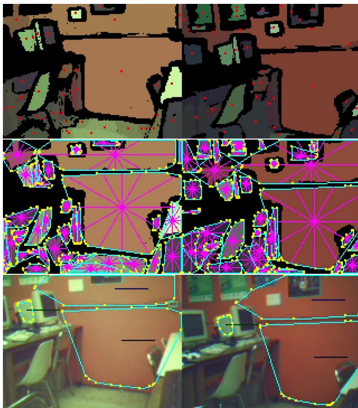
Fig. 2. Segmented regions (top), with convex hulls plotted and distance lines from the centroid added (middle). Stereo-matched regions (bottom) are bounded by a colored box, with a line emanating from the centroid of the image.
