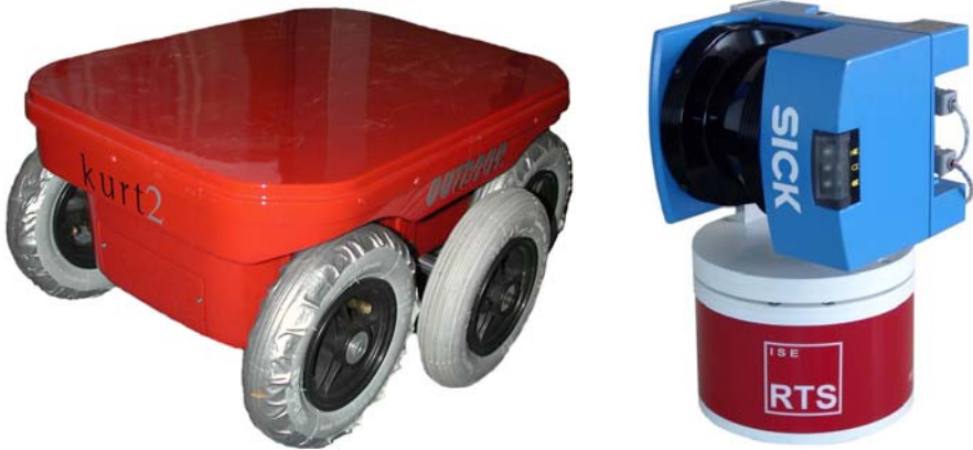
Fig. 1. The mobile robot platform Kurt3D offroad (left) and the 3D laser scanner (right) The scanner rotates around the vertical axis. It's technical basis is a SICK 2D laser range finder (LMS-200).
