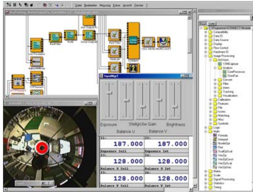
Fig. 5. ICONNECT GUI with signal graph (top), visualization of sensor data (left), a user cockpit (center) and the module library (right)
