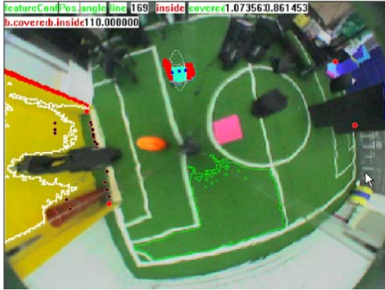
Fig. 5. Grown regions which fail to meet the validation criteria. Pixels of the goal-box and ball regions are outside the expected region, or the field region does not cover a required percentage of the expected region.
