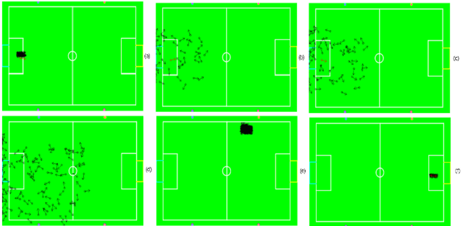
Fig. 4. (a) Just after being kidnapped, (b) first frame after kidnapping, (c) after 2 frames, (d) after 3 frames, (e) after 4 frames, and (f) after 11 frames the robot finds its position
