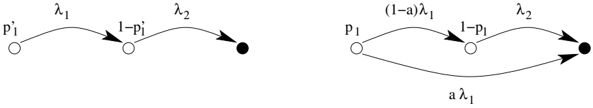
Fig. 2. The canonical representation of second-order PH distributions (left) and its transformation (right)
