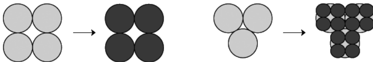
Fig. 2. Mappings of orthogonal (on the left) or hexagonal (on the right) grids into an orthogonal grid
