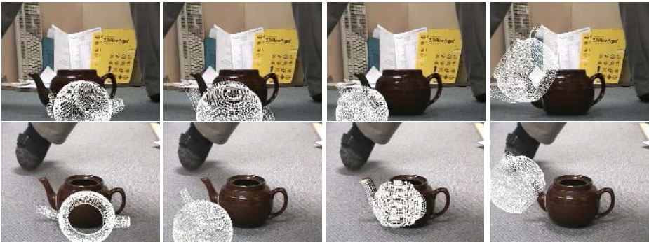
Fig. 6. Example rotations, which still converged using the ICP+OF algorithm but failed with ICP alone
