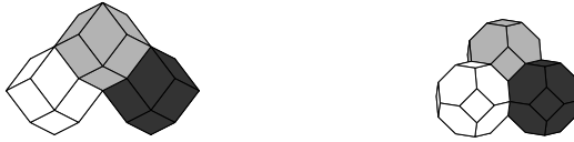
Fig. 1. The light grey voxel is 1-neighbour to the dark grey voxel. The white and light grey voxels are 2-neighbours to the dark grey voxel. Left: fcc, right: bcc.
