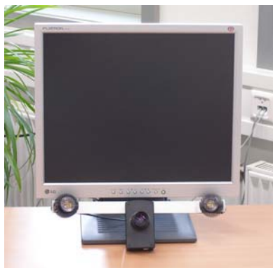
Fig. 1. Physical setup of the eye tracking hardware, consisting of a single high-resolution camera below the display and two infrared LEDs to either side of the camera
