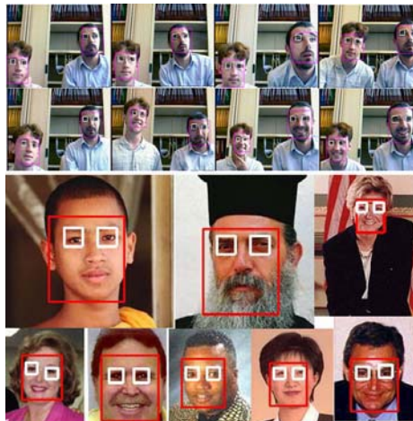
Fig. 9. Face detection and Eye tracking result on a subset of the images database
