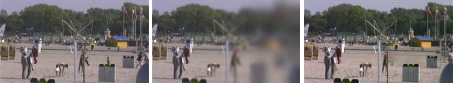
Fig. 1. Example of our spatio-temporal filtering algorithm. The effects in the middle and the right pictures can be combined in an arbitrary manner. Gaze position is indicated by the little white square to the left (below the white sail). Left: Still shot of the original movie. Middle: Spatial blur that is increased towards the visual periphery. Right: Temporal blur. Note the disappearance of the little girl to the right.
