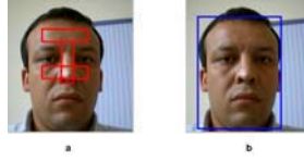
Fig. 3. (a) Skin colour is initialized in the area E, (b) face detection with CFF+skin colour
