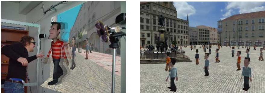
Fig. 1. Left: The user controls his navigation by bending his body. Wireless tracking is performed with infrared cameras to enable an unobtrusive interface. Right: Crowd simulation is done by enabling emergent behaviour of each character.
