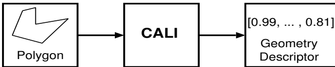
Fig. 2. Block diagram for computing the geometric descriptor
