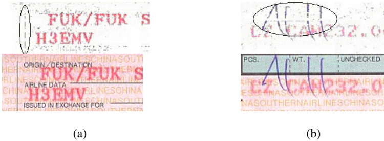
Fig. 1. (a) The obvious error in pixels classification; (b) Incorrect pixels classification for unknown color class. In the upper: object pixels; In the lower: the original image; Within the ellipse: incorrect object pixels.
