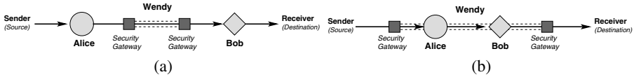
Fig. 15. Location of Alice, Bob, and Wendy under and IPsec Tunneling Mode. (a) Alice and Bob embed and extract, respectively, covert data outside the tunnel; Wendy is within the tunnel, so an attempt to modify the traffic might cause the authentication to fail. (b) Alice, Bob, and Wendy are all inside the tunnel; the warden can prevent covert channels in the outer header.
