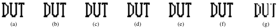
Fig. 5. The original watermark image and extracted watermark images under various conditions. (a) original watermark image. (b) extracted watermark image without any attack. (c) mp3 compression. (d) cropping. (e) lowpass filtering (cut off frequency is 16kHz). (f) resampling (from 44.1k to 88.2 kHz, then to 44.1 kHz). (g) adding white Gaussian noise (SNR is 21dB).
