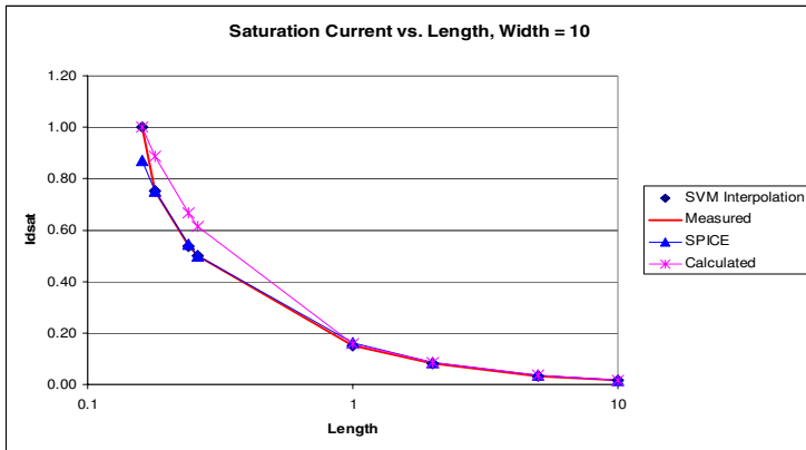
Fig. 1. Saturation Current Length Scaling (RBF SVM, SPICE, & Calculation)
