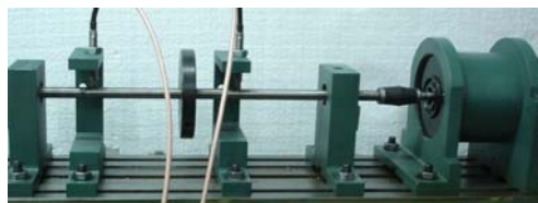
Fig. 2. A single-span-single-disc (jeffcott) rotor system
