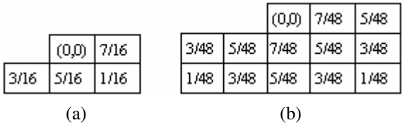
Fig. 1. Two kinds of error diffusion filters: (a) is Steinberg filter, and (b) is Jarvis filter
