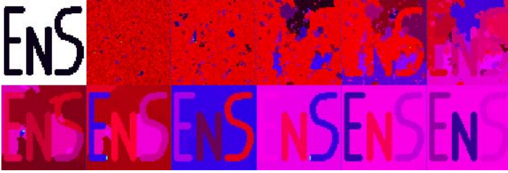
Fig. 1. The original picture followed by the different steps of its segmentation by the algorithm of Campbell, Wang and Jayaprakash
