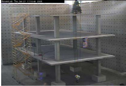
Fig. 2. An instrumented test infrastructure at the Bowen Labs (three story 30' \times 50' structure) with extensive actuation and response testing capability
