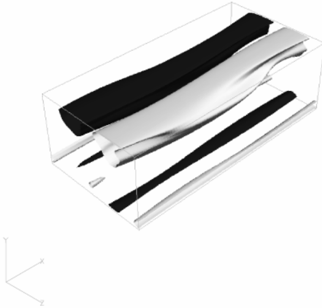
Fig. 3. Surfaces of constant x -velocity reconstructed from the first five POD modes at t^* = 72
