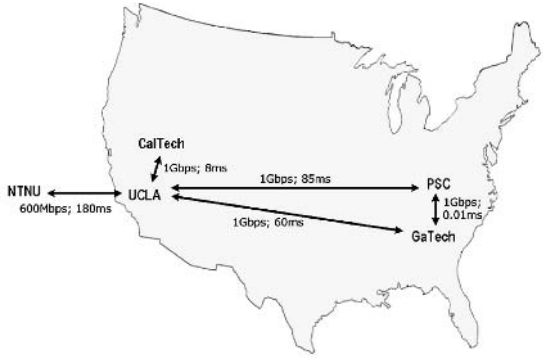
Fig. 5. Topology and path properties (bottleneck capacity and round trip delay) of selected gigabit Internet paths
